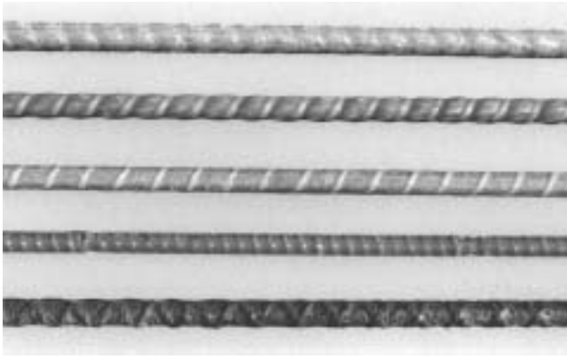
Fig. 2.1—Commercially available GFRP reinforcing bars.
